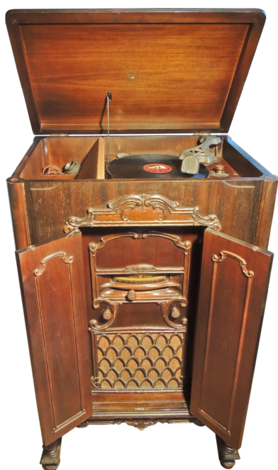
Fig 10: RCA Victor Radio Electrola Model RE-57. Its microphone can be seen in the left compartment next to the record player.
